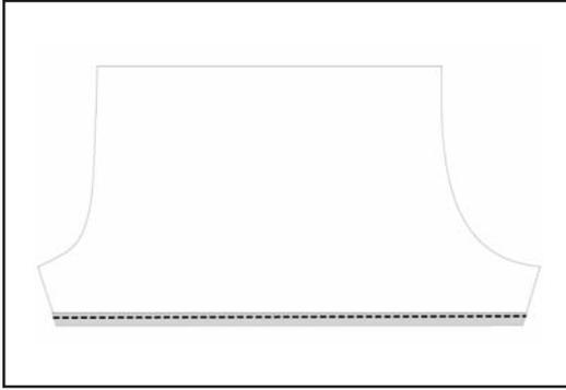
1. Turn & press a 1/4" hem along the bottom edge of each Bloomer piece, RST. Repeat, and topstitch in place for a rolled hem.
