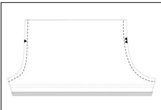
4. Pin & sew the Bloomer pieces together, Right Sides facing, along their curved grain seams. Make sure to line up the single (front seam) & double (back seam) notches.
